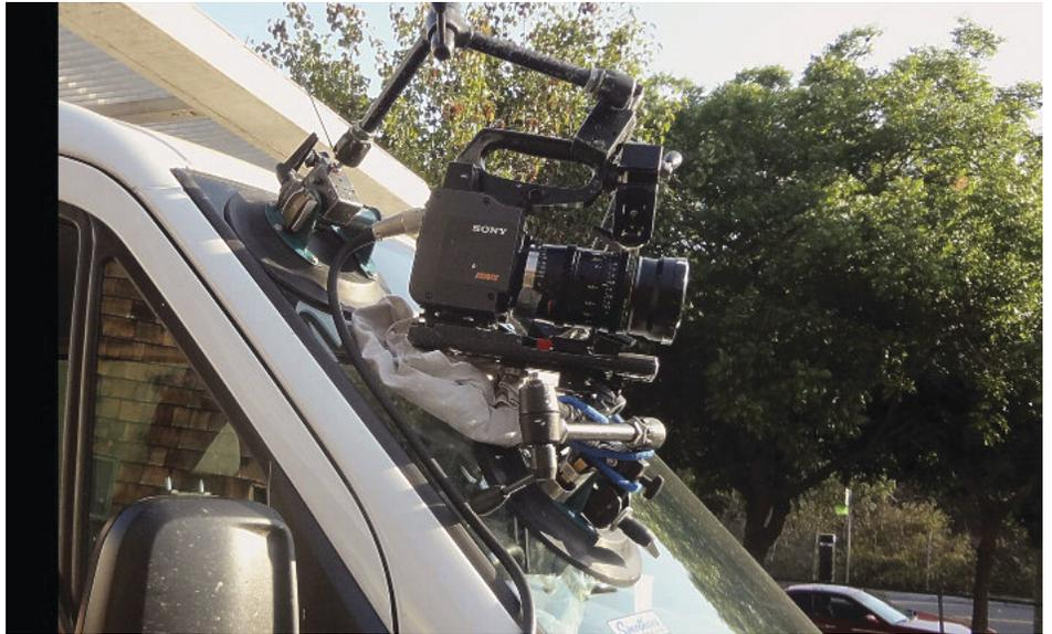
Camera on front of van at bus driver's eye level – driven along bus path – to capture base video used to construct video-in-video visibility study.
